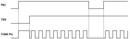
Fig. 8. TONE Output Pin Timing Chart
